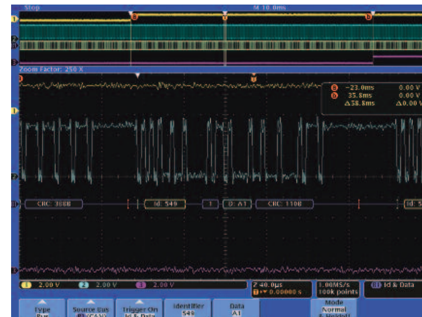
Automatically decode serial bus information in correlation to the live signal in an easy to read format
