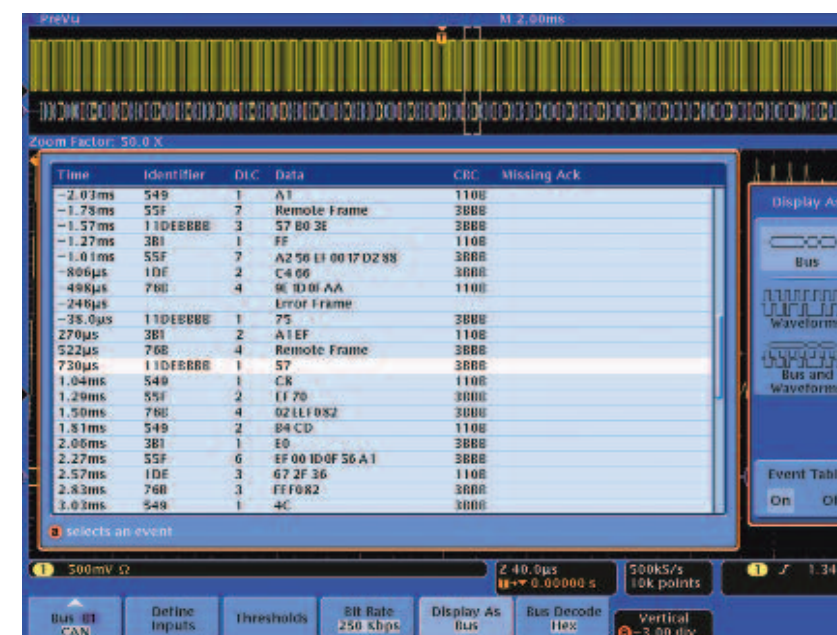
Capture long record lengths and analyze specific bus events in an event table listing
